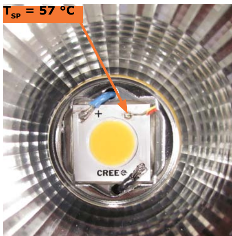
Figure 9: CXA1507 PAR30 T_{SP} measurement with thermocouple
